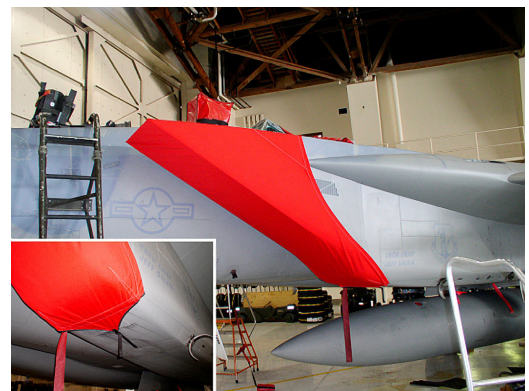
Intake Cover, Attachment Detail (inset)
