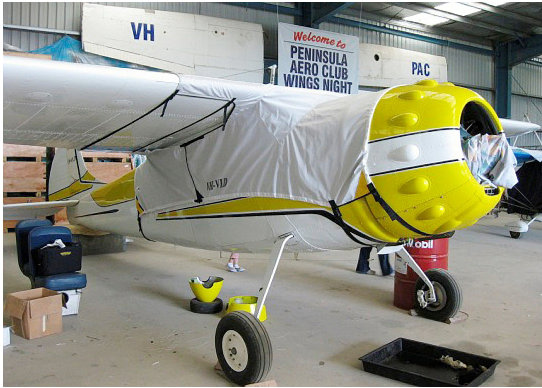
Cessna 195 Canopy Cover, over-top, 24" fwd ext to cover cowl ring gap, gas cap ext. Cessna 195 Over-Top Canopy, Engine & Prop Covers
