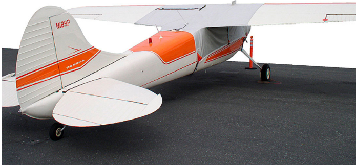
Cessna 195 Over-Top Canopy, Engine & Prop Covers
