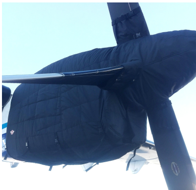
ATR-72-202 Insulated Engine & Prop Hub Covers
