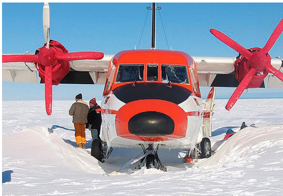
Casa 212 Insulated Engine & Propellor/Spinner Covers
