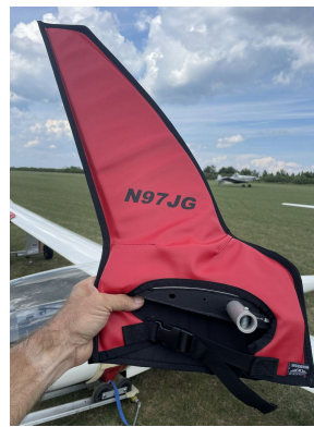
Schempp-Hirth Ventus-2B winglet/wingtip pads
