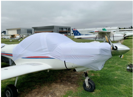
Grob 115 Canopy/Engine Cover, test fit cover
