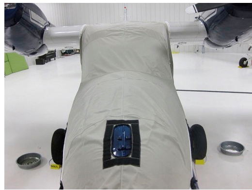
Grumman Widgeon Cockpit/Nose Cover, tie-down cleat detail
