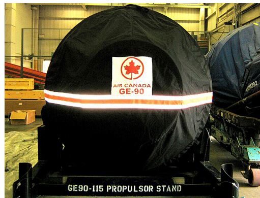
GE90-115 Propulsor QEC Engine Long-term Storage/Transport Cover "Bag" Boeing 777
