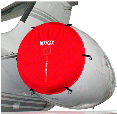
Bombardier Global Express Intake Covers Intake/Exhaust Covers, 3-Strap Type. Successfully installed by two crew, one ladder.
