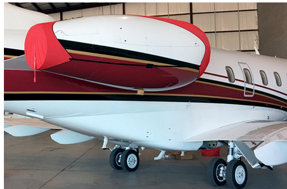
Bombardier Global Express Intake Covers Intake/Exhaust Covers, 3-Strap Type. Successfully installed by two crew, one ladder.
