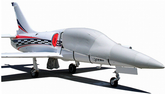
L39 Canopy/Nose Cover & Intake Plugs
