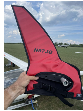
Schempp-Hirth Ventus-2B winglet/wingtip pads
