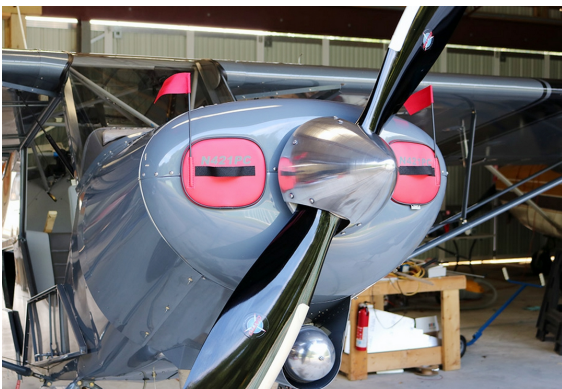
Piper PA-18 Super Cub Engine Inlet Plugs
