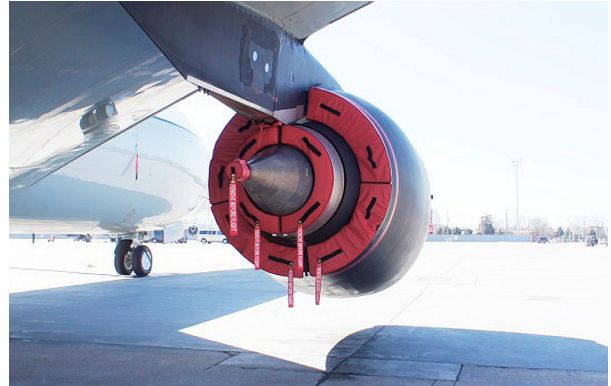
RC-135W Bypass Vent and Exhaust Plugs
