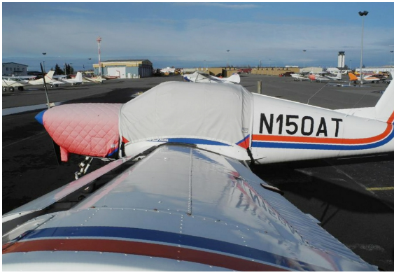
Koliber 150A Canopy Cover, Insulated Engine Cover
