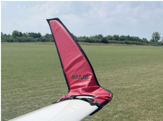
Schempp-Hirth Ventus-2B winglet/wingtip pads
