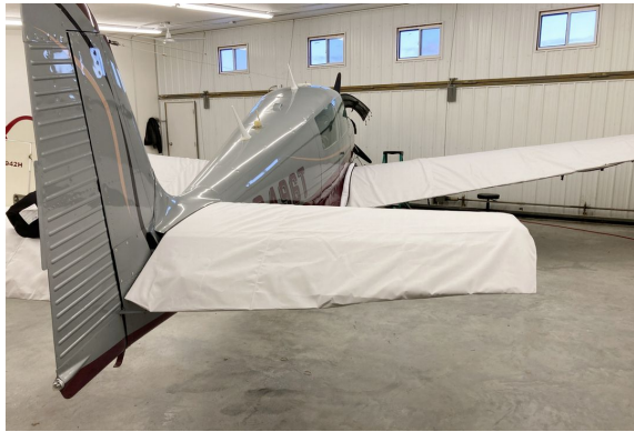
Navion Rangemaster Wing & Horizontal Stabilizer Covers
