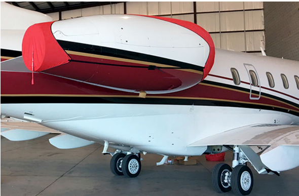
Canadair Challenger 300 Intake/Exhaust Covers, 3-Strap Type Intake/Exhaust Covers, 3-Strap Type. Successfully installed by two crew, one ladder.
