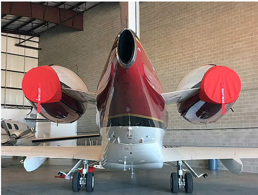
Canadair Challenger 300 Intake/Exhaust Covers, 3-Strap Type Intake/Exhaust Covers, 3-Strap Type. Successfully installed by two crew, one ladder.
