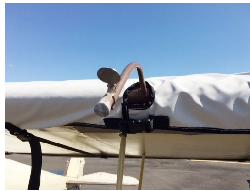
Luscombe 8A-8F Silvaire Wing Covers, Pitot Tube detail.
