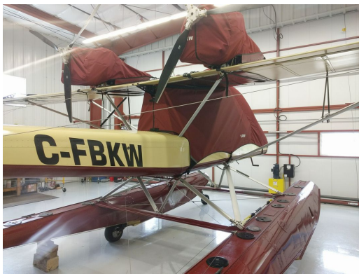
Lockwood AirCam Canopy Cover (fully enclosed bubble), Engine Covers
