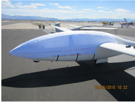
DG-505 Canopy/Nose Cover (test fit cover)
