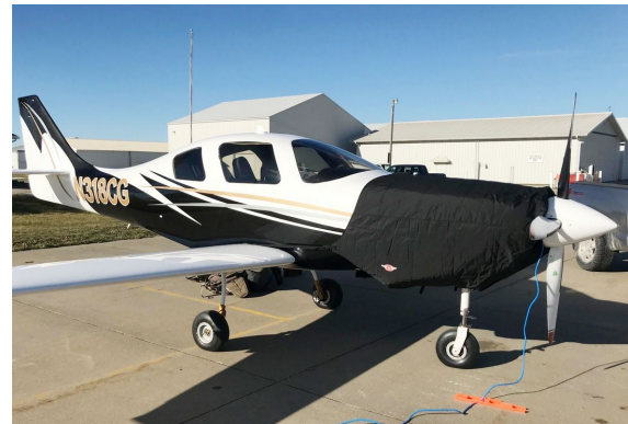
Lancair IV-P Insulated Engine Cover, fully enclosed
