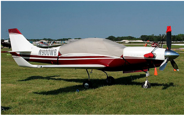
Lancair IV Canopy Cover & Prop Tie/Exhaust Cover
