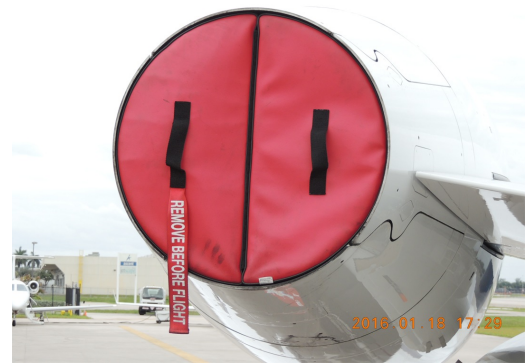
Embraer Legacy 500 Engine Exhaust Plug, folding type
