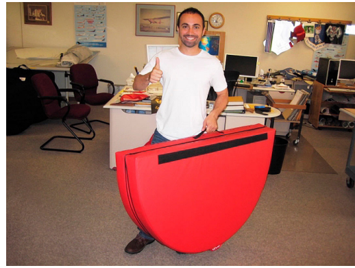
Boeing 737 FOD protection Intake Plug, folding type
