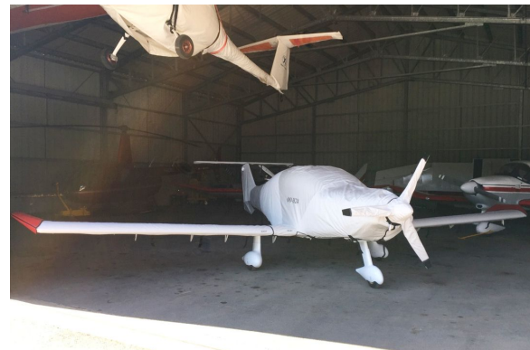
Dynaero MCR.4 Pickup Complete Cover Set.
