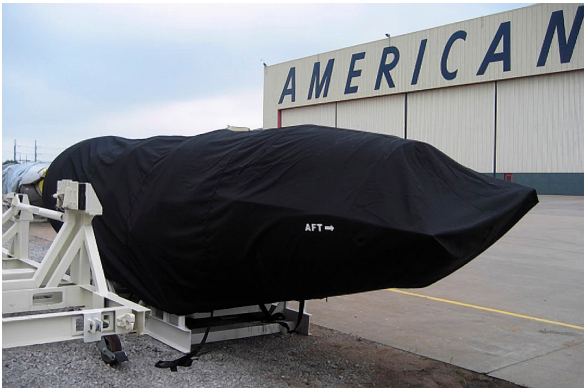
PW JT8D Off-Link Protective Long-term Storage "Rain Cap" Engine Cover
