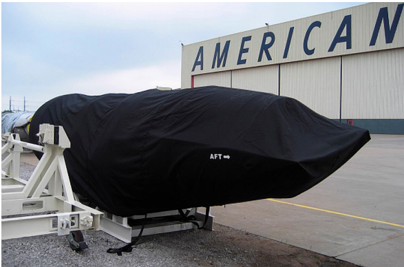
PW JT8D Off-Link Protective Long-term Storage "Rain Cap" Engine Cover PW JT8D Off-Link Engine Storage Cover w/ Nose Cowl & TR's, "Rain Cap" style
