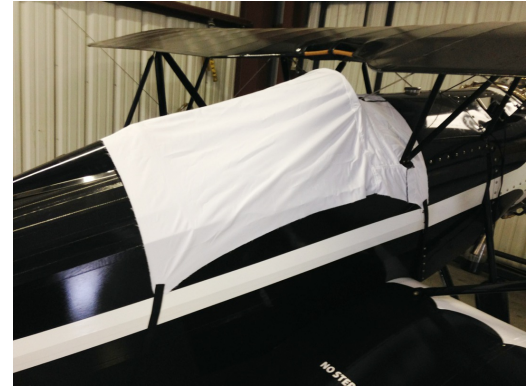
Rose Parrakeet Canopy Cover (test fit cover)
