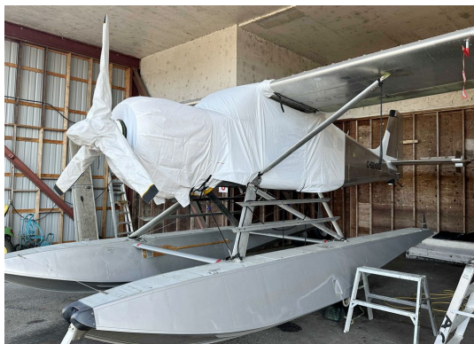
Murphy Moose Extended Canopy Cover, Engine & Prop Covers, test fit covers.
