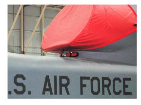
Intake Cover with small inlet plug
