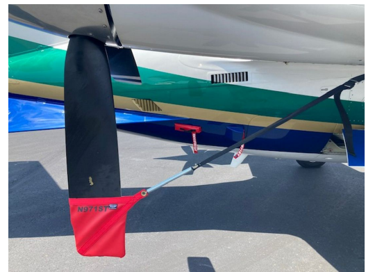
Piaggio P180 Prop Ties
