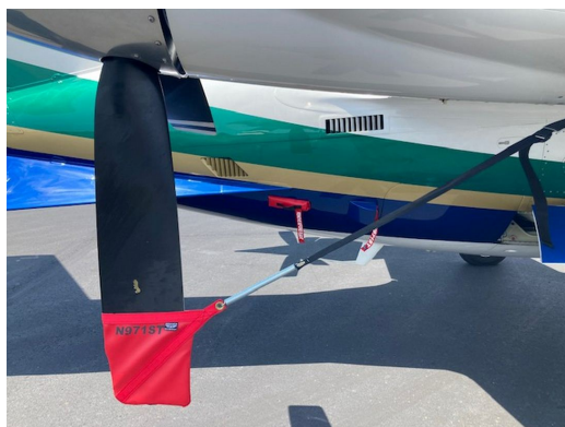
Piaggio P180 Prop Ties
