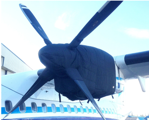
ATR-72-202 Insulated Engine & Prop Hub Covers
