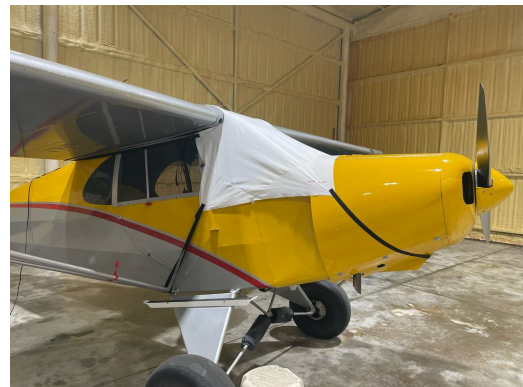
Piper J5A Windshield/Skylight Cover, test fit
