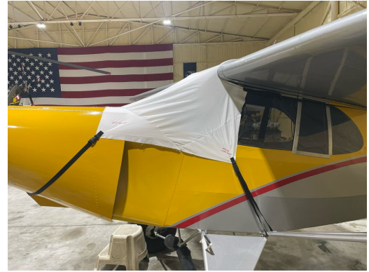
Piper J5A Windshield/Skylight Cover, test fit
