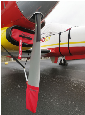
Piper PA-42 Cheyenne III Prop Tie/Exhaust Cover, Inlet Plugs
