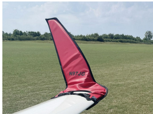
Schempp-Hirth Ventus-2B winglet/wingtip pads
