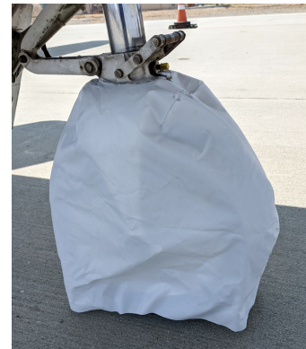
CJ1 Nose Gear Tire Cover, test fit
