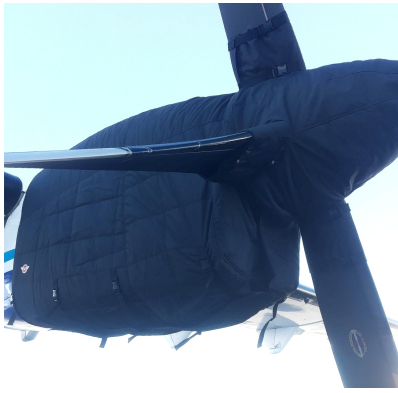
ATR-72-202 Insulated Engine & Prop Hub Covers
