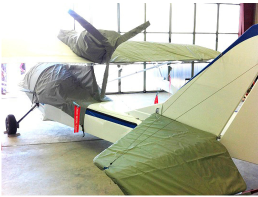
SeaRey Canopy, Engine, Wing & Horizontal Stab. (test fit covers)
