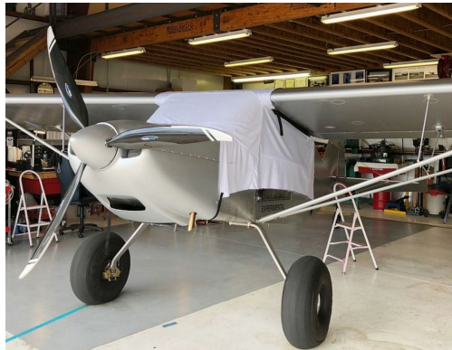
Rans S-20 Canopy Cover, test fit cover
