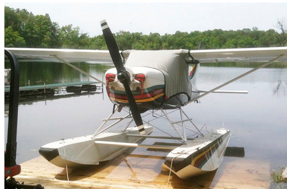
Glastar Sportsman Canopy Cover and Engine Plugs
