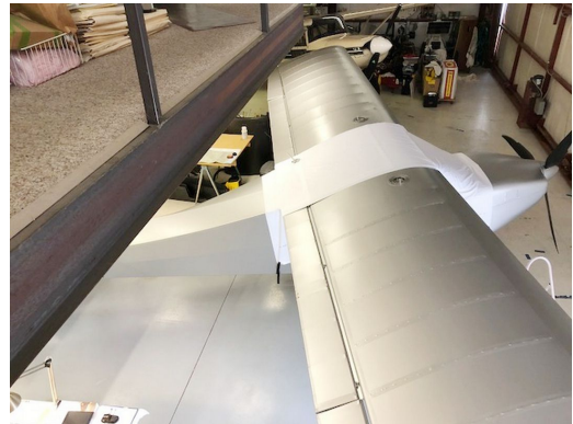
Rans S-20 Canopy Cover, test fit cover
