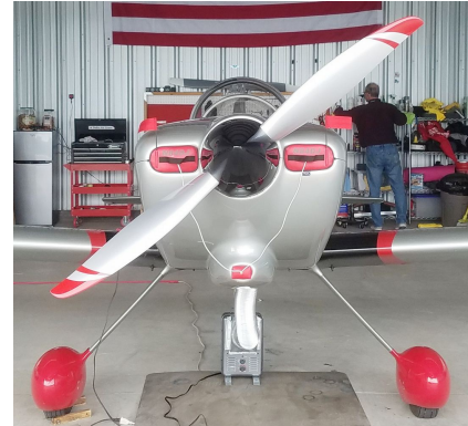
Van's Aircraft RV-8/8A Engine Inlet Plugs
