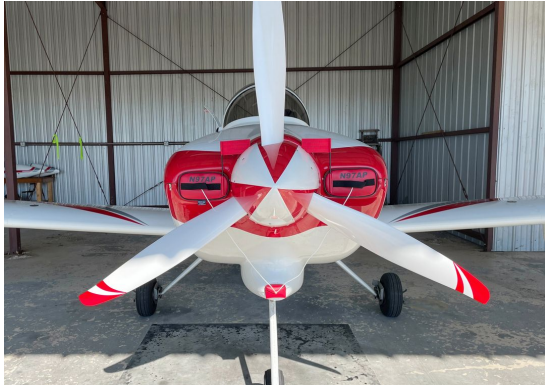
Van's RV-8 Engine Inlet Plugs
