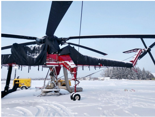
Sikorsky S-64 Skycrane, CH-54 Tarhe Insulated Engine, Rotor Sikorsky S-64 Canopy/Nose, Engine Area, Blade, Rotor, Tail Rotor Hub, Tailboom, Stabilizer & Tail Rotor Covers Sikorsky S-64 Canopy/Nose, Engine Area, Blade, Rotor, Tail Rotor Covers (illustration)
