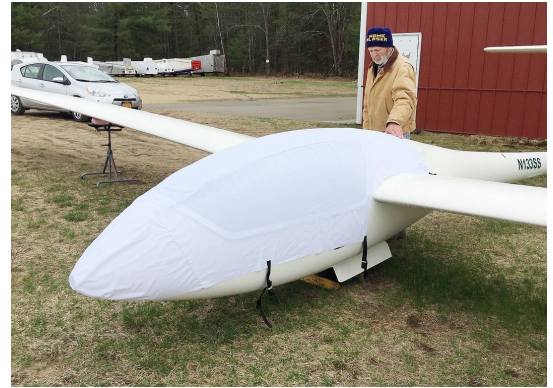
Grob 102 Astir CS Canopy/Nose Cover (test fit)
