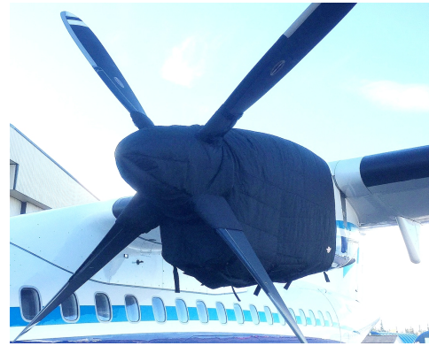
ATR-72-202 Insulated Engine & Prop Hub Covers
