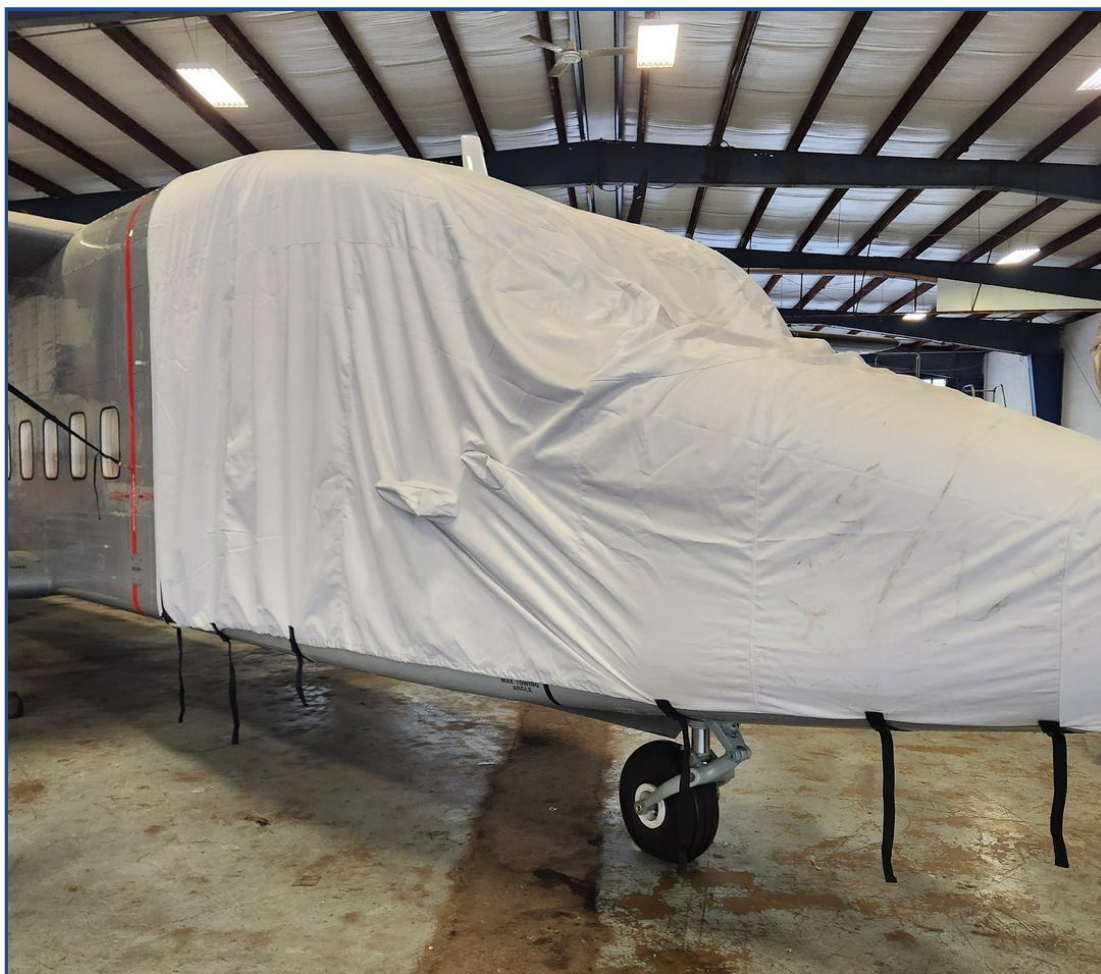
Short Skyvan Forward Fuselage/Nose Cover
