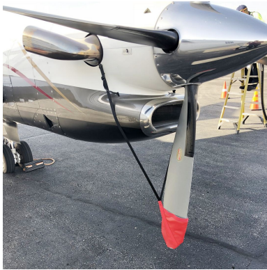
Beech King Air 350 Prop Tie-Downs
