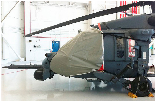
Sikorsky UH-60 Intake/Exhaust Cover Set (IR suppressors)
