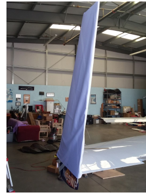
Velocity Vertical Stabilizer Covers, test fit cover
