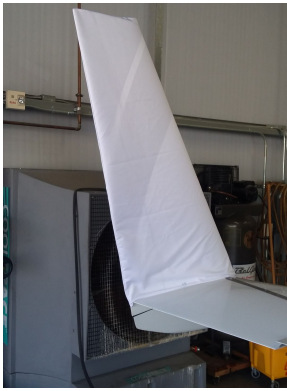
Velocity Vertical Stabilizer Covers, test fit cover
