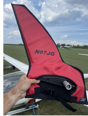
Schempp-Hirth Ventus-2B winglet/wingtip pads
