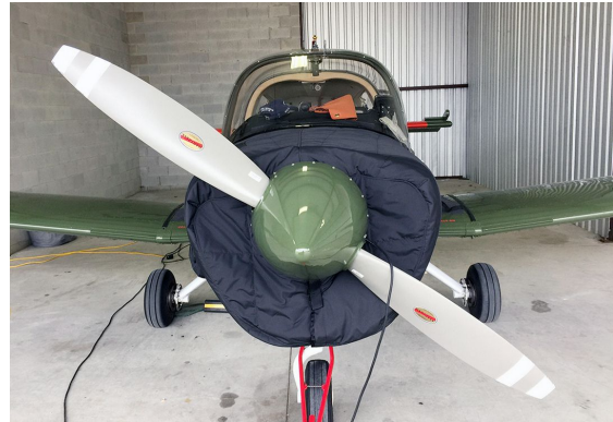
Scottish Aviation Bulldog Insulated Engine Cover
