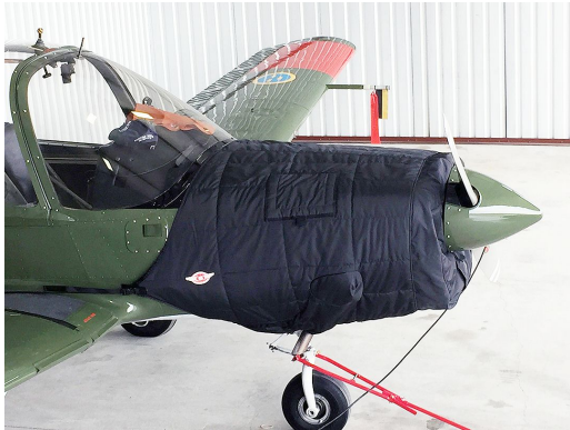
Scottish Aviation Bulldog Insulated Engine Cover
