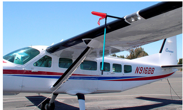
Cessna 208 Caravan Telescoping Pitot (for amphib. models)
