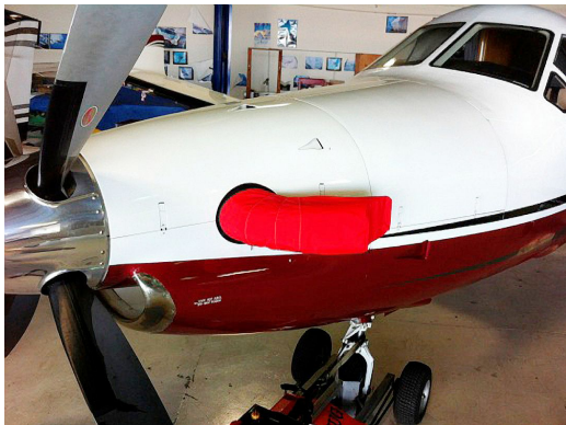
Pilatus PC-12 Exhaust Cover, Fully Enclosed, for protection against corrosion.
