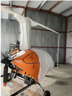
Celier Argon 915 Canopy/Nose Cover, Rotor Mast Cover, test fit covers
